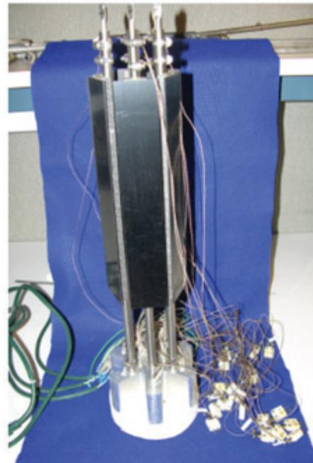
*Figure 1. Thermosyphon setup bonded with silver-doped EP30HT-LO and used to assess the generation of non-condensable gases by irradiating water with gamma radiation.*
